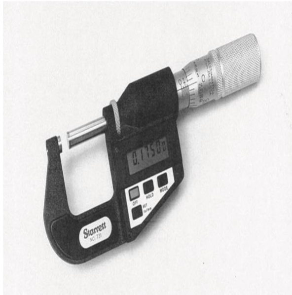
(a) External micrometer
