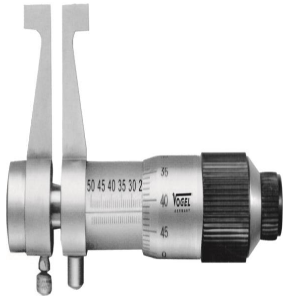
(b) Internal micrometer
